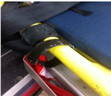
Fig 1d: Undo Velcro on aerolite stretcher to make room for base plate latching
