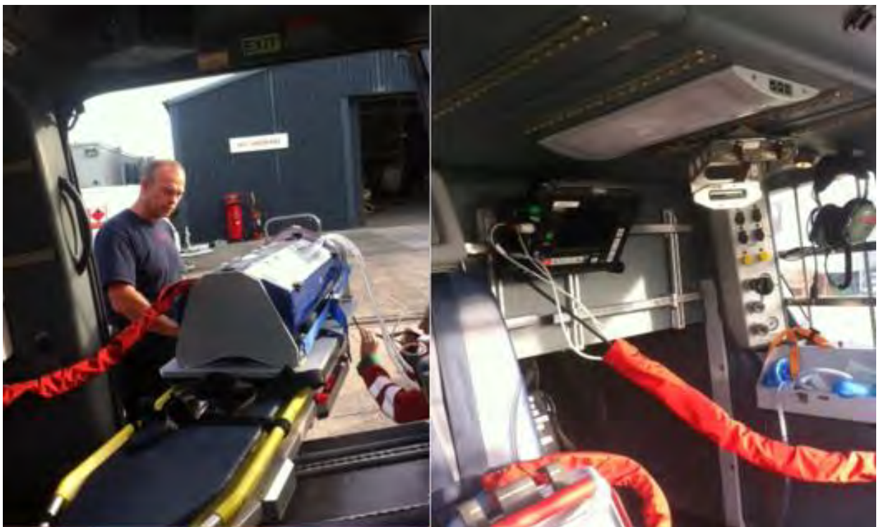
Fig 3c/d: Move monitor to bracket, then start sliding stretcher home. Ventilator/oxygen has shorter tubing, so has to follow Babypod until stretcher far enough in to transfer vent/O2 to helicopter.
